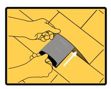
2. Remove the paper and insert the patch under the shingle. Orient the patch metal side up, with the butyl strip toward the shingle's broken adhesive seal.
