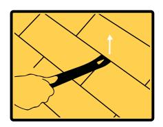
1. Locate the hole and break the adhesive seal on the shingle course just wide enough to fit the 4-inch wide QuickPATCH®.
