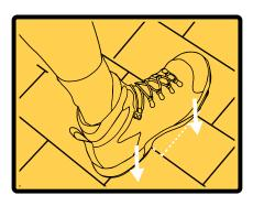
**4.** Press the shingle course back down. Then, step on and press the patch area with even pressure to engage the butyl and reseal the adhesive STRIP.
