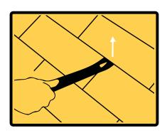
Locate the hole and break the adhesive seal on the shingle course just wide enough to fit the 4-inch wide QuickPATCH™.
