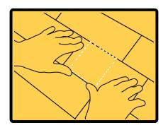
**3.** Push the patch under the shingle until it covers the hole and sits flush with the bottom edge of the shingle course.
