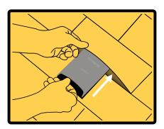
2. Remove the paper and insert the patch under the shingle. Orient the patch metal side up, with the butyl strip toward the shingle's broken adhesive seal.
