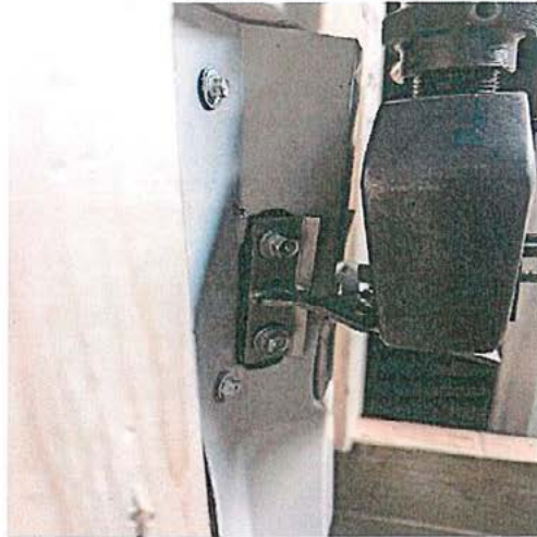
The L-Foot bent until no more loading could be achieved
