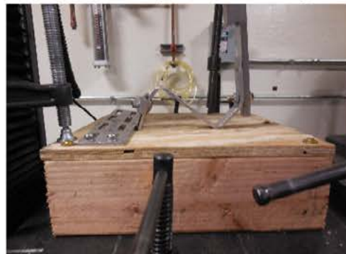
Photo 8: Typical Failure - Contact with Plywood
