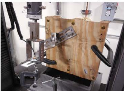
Photo 11: Deformation of Hook at Weld
