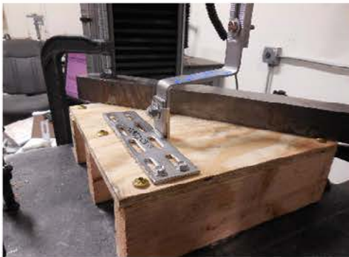
Photo 5: Compression Test Setup
