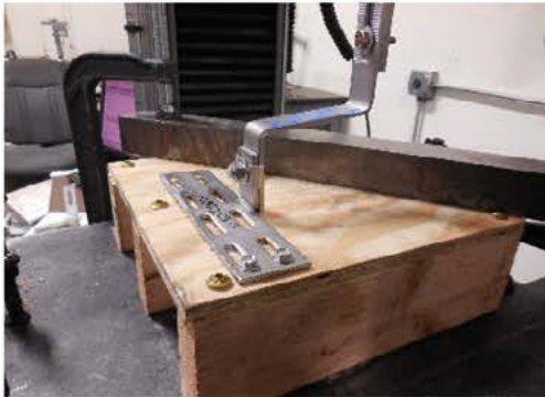
Photo 5: Compression Test Setup
