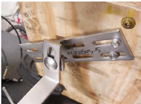
Photo 12: Typical Failure Mode - Deformation at Weld
