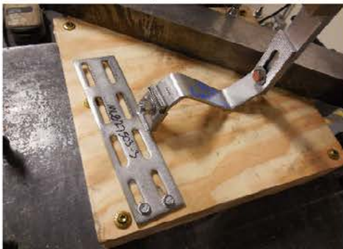
Photo 7: Hook Contact with Plywood
