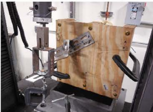
Photo 11: Deformation of Hook at Weld
