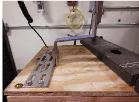
Photo 6: Compression Test Setup
