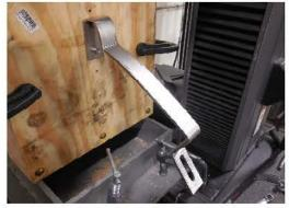
Photo 11: Deformation of Hook at Base
