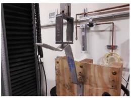
Photo 10: Adjusted Test Setup to Accommodate Flexure
