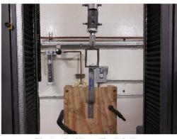
Photo 9: Shear Test Setup
