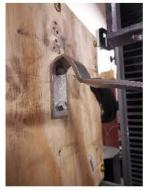
Photo 12: Typical Failure Mode - Deformation at Base
