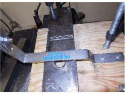
Photo 2: Tensile Test Setup
