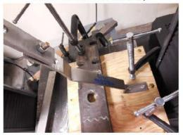
Photo 3: Typical Failure Mode - Fastener Pullout
