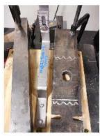
Photo 5: Compression Test Setup
