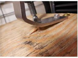
Photo 4: Closeup of Fastener Pullout
