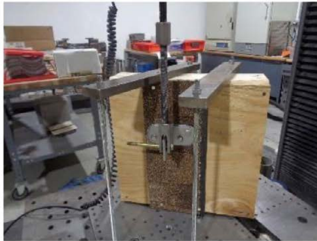
Photo No. 7 ASTM D7147 - Configuration F2 Test in Progress
