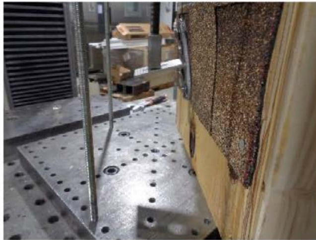
Photo No. 5 ASTM D7147 - Configuration F3 Test in Progress
