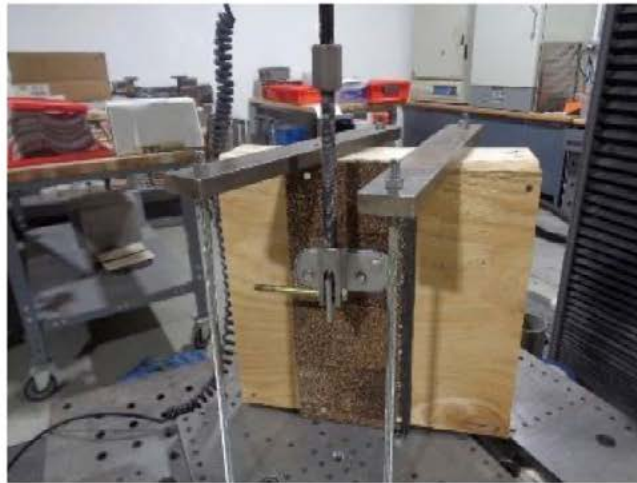
Photo No. 7 ASTM D7147 - Configuration F2 Test in Progress
