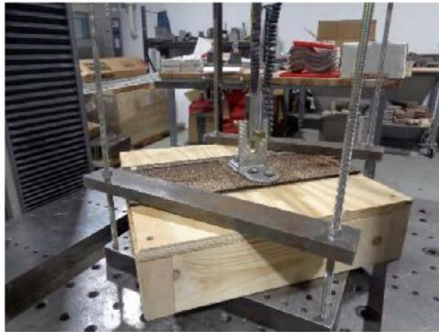
Photo No. 9 ASTM D7147 – Configuration F1 Vertical Load Test Setup
