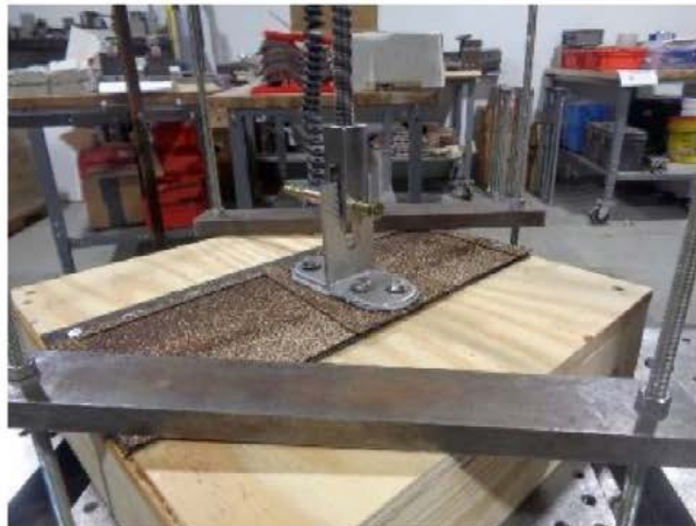
Photo No. 10 ASTM D7147 – Configuration F1 Vertical Load Test in Progress
