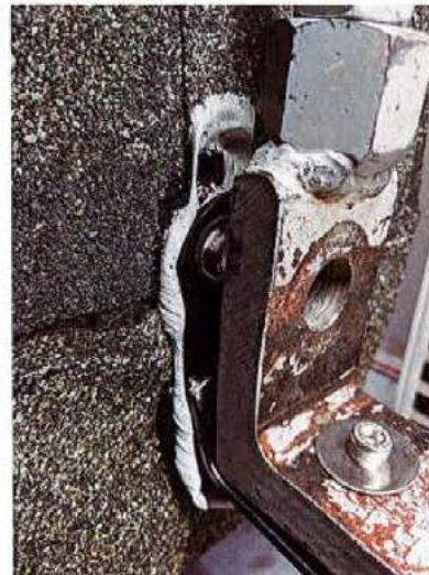
Figure 4c. Bolt failure mode.
