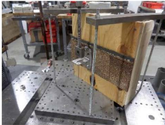
Photo No. 3 ASTM D7147 - Configuration F3 Test Setup
