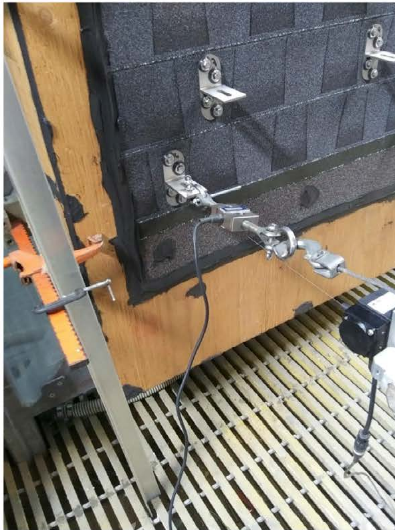
Photo No. 1 Pullout Test
