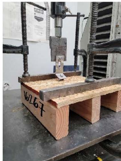
Figure 1b. Typical failure mode.
