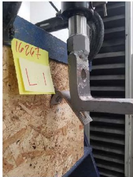
Figure 2b. Typical failure mode.
