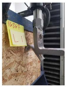
Figure 2b. Typical failure mode.
