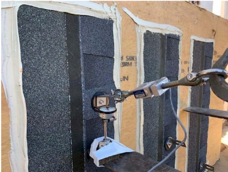
Photo No. 1 Pullout Test
