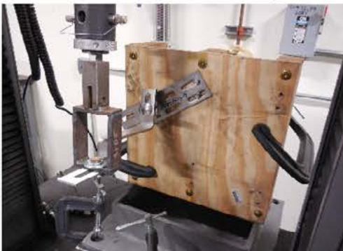
Photo 11: Deformation of Hook at Weld
