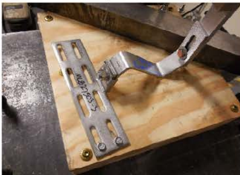
Photo 7: Hook Contact with Plywood
