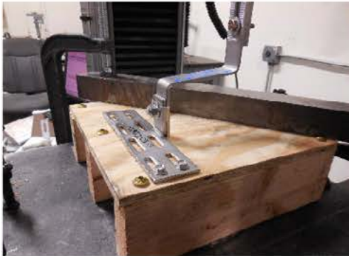
Photo 5: Compression Test Setup
