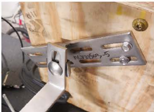
Photo 12: Typical Failure Mode - Deformation at Weld
