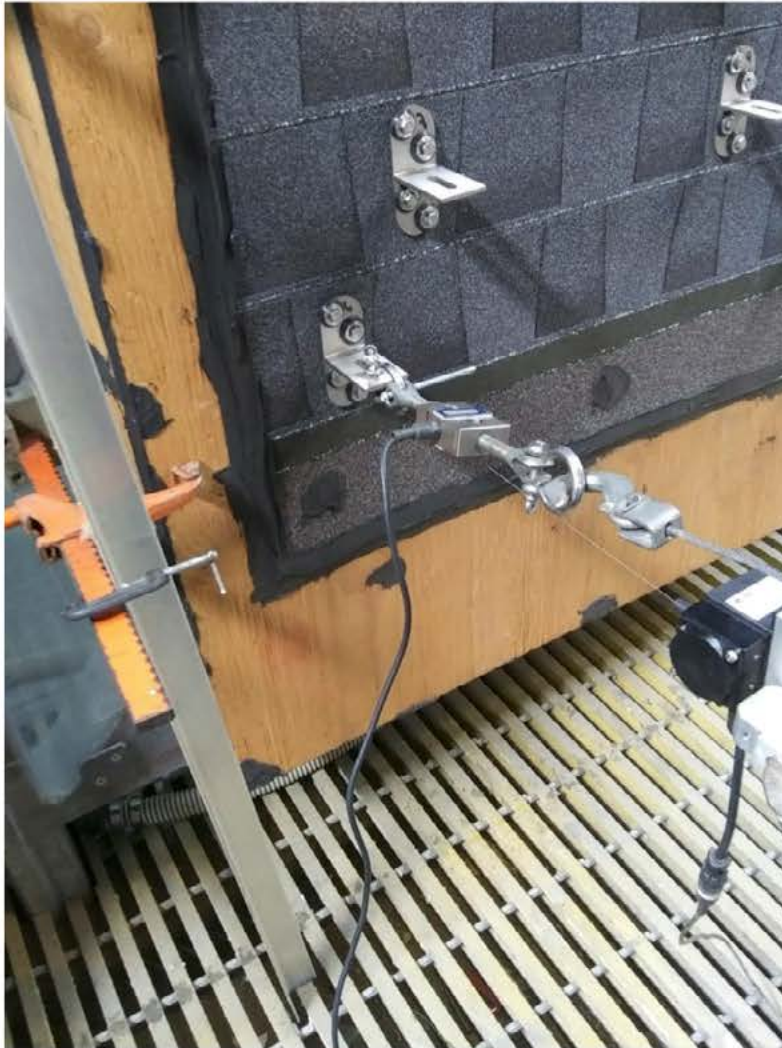
Photo No. 1 Pullout Test
